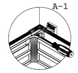
1- Loosen to screws on corner plastic. Adjust according to frame of drawer measurements of the width the module (A-1).
