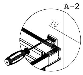
2- Fix to frame of drawer front 10 mm inside from connection plastics on module (A-2).
