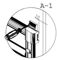
1- Fix to mechanism of shoes at a distance of 10 mm in front of the module from connection plastic in module (A-1).
